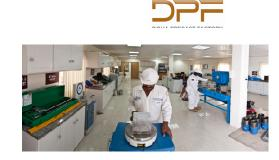
Doha precast Factory has the Laboratory accredited by IAS for ISO IEC 17025 for most of the parameters (34) related to Aggregate test, Concrete Test and Concrete Pipe test as per BS and ASTM as required by QCS 2014
